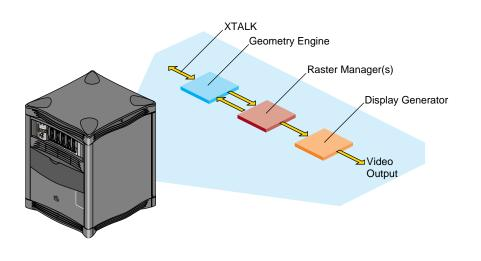
Figure 5. Onyx2 Visualization Pipeline
