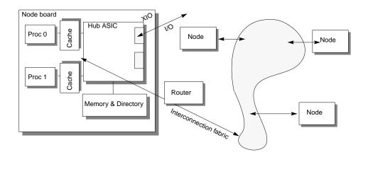
Figure 27. Location of a Router Board in an Onyx2 System
