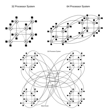
Interconnection fabric: multidimensional. Many connections can be made at a time. R=Router Black squares = Node with one or two CPUs
