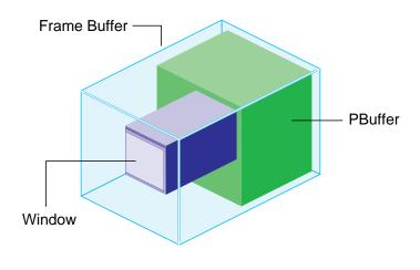
Figure 16. Disjoint Buffers and PBuffers
