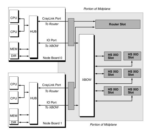
Figure 25. Functional Location of XBOW ASIC
