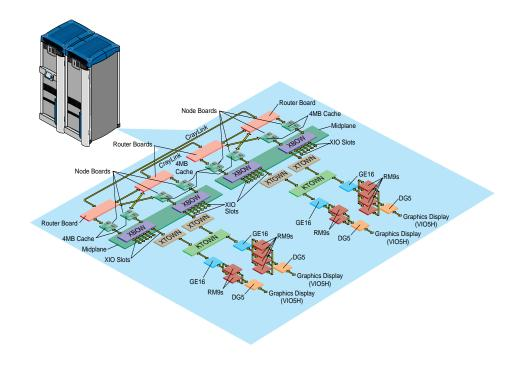
Figure 4. Onyx2 InfiniteReality2 Multi-Rack System
