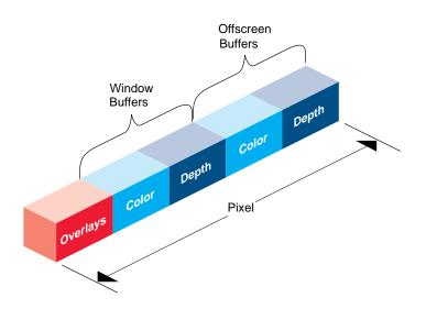
Figure 15. Frame Buffer Pixel Memory Including Offscreen Buffers
