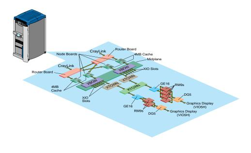
Figure 3. Onyx2 InfiniteReality2 Single-Rack System
