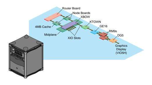
Figure 2. Onyx2 InfiniteReality2 Deskside System
