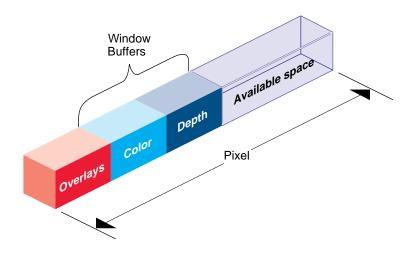
Figure 14. Frame Buffer Pixel Memory
