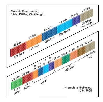
Figure 7. Choices of Allocation of 256 Bits of Frame Buffer Memory
