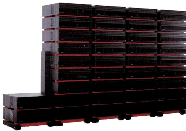
Figure 2-4: A 4x8 Scali system boxed in Scali cabinets
