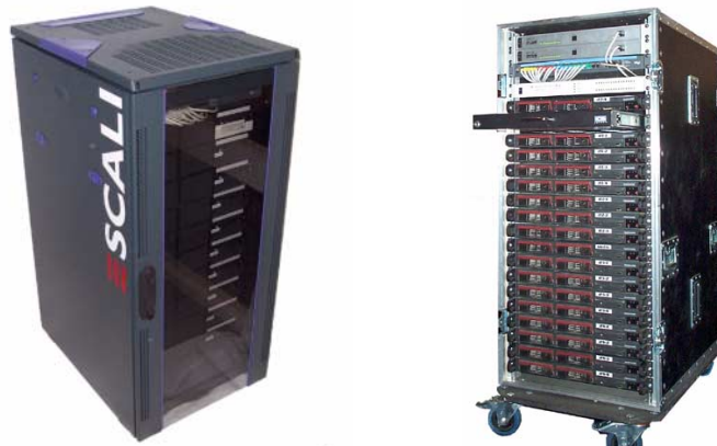
Figure 2-2: Scali system cabinet examples: Standard half-size Terarack (left) and a ruggedized version for portable supercomputing (right)
