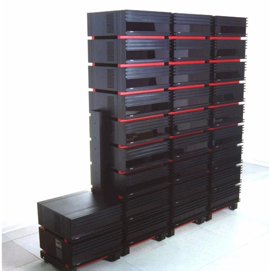
Figure E-1: The Scali system cabinet
