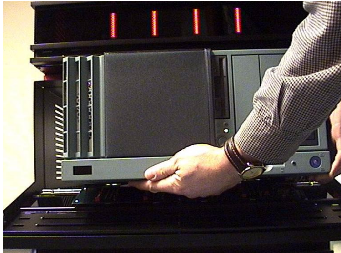
Figure E-9: Insertion of node in enclosure
