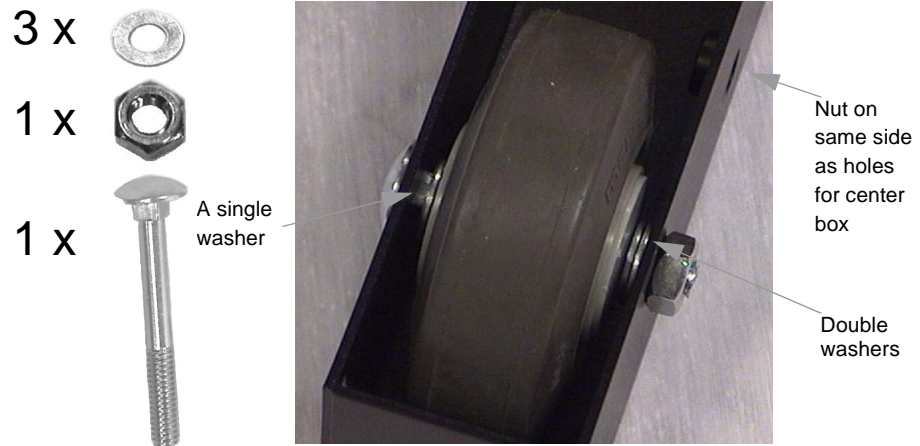
Figure E-3: Assembly of the casing wheels
