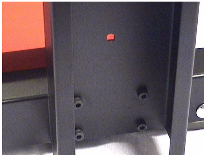
Figure E-4: Assembling backbone to the base
