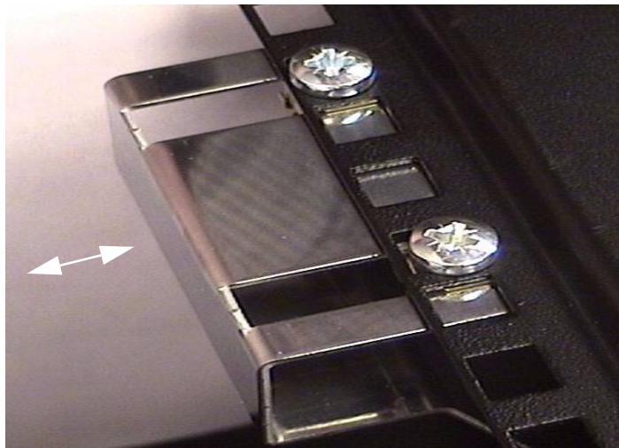
Figure E-10: Node guide adjustment
