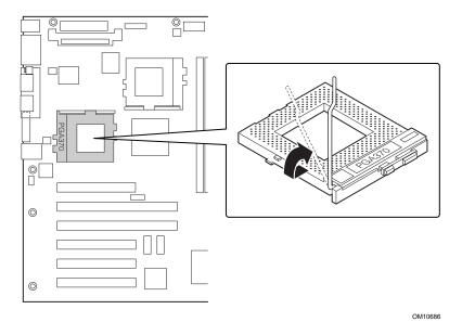
Figure 4. Raise the Locking Bar
