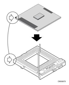
Figure 5. Insert the Processor
