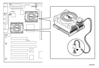
Figure 9. Connect the Processor Fan
