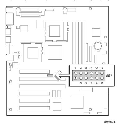
Figure 10. Processor Clock Speed Jumper
