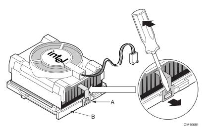
Figure 8. Attach the Heatsink
