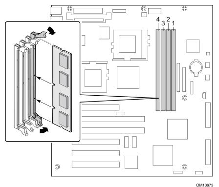
Figure 3. Installing DIMMs
