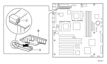
Figure 12. Installing a VRM
