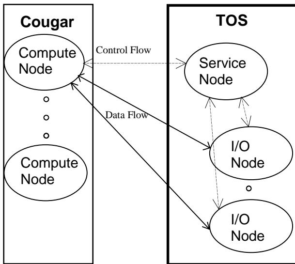
**Figure 5: I/O service process control and data flow**
