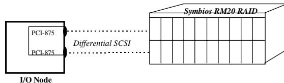
**Figure 8: Symbios RAID connection to TFLOPS system**
