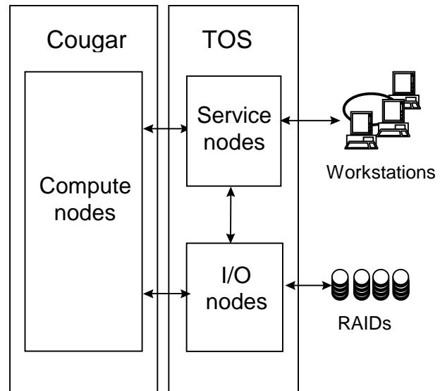
**Figure 1: Overview of the TFLOPS system architecture**
