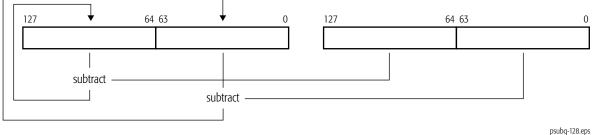
This instruction operates on both signed and unsigned integers. If the result overflows, the carry is ignored (neither the overflow nor carry bit in rFLAGS is set), and only the low-order 64 bits of each result are written in the destination.
