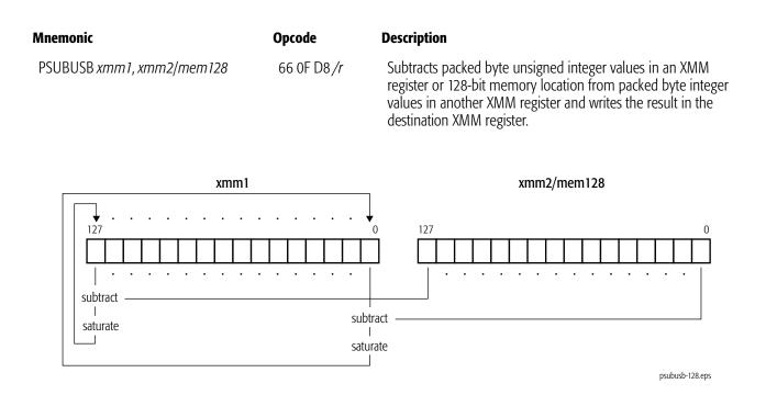
For each packed value in the destination, if the value is larger than the largest unsigned 8-bit integer, it is saturated to FFh, and if the value is smaller than the smallest unsigned 8-bit integer, it is saturated to 00h.
