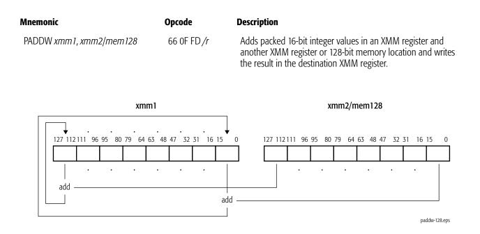
This instruction operates on both signed and unsigned integers. If the result overflows, the carry is ignored (neither the overflow nor carry bit in rFLAGS is set), and only the low-order 16 bits of the result are written in the destination.
