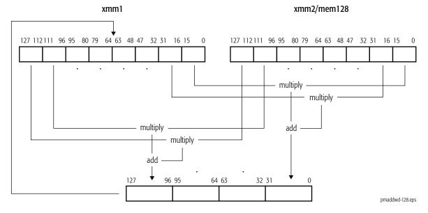
There is only one case in which the result of the multiplication and addition will not fit in a signed 32-bit destination. If all four of the 16-bit source operands used to produce a 32-bit multiply-add result have the value 8000h, the 32-bit result is 8000\_0000h, which is incorrect.
