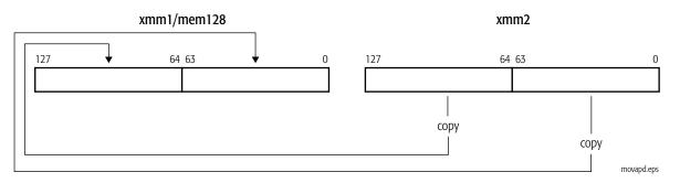
A memory operand that is not aligned on a 16-byte boundary causes a generalprotection exception.
