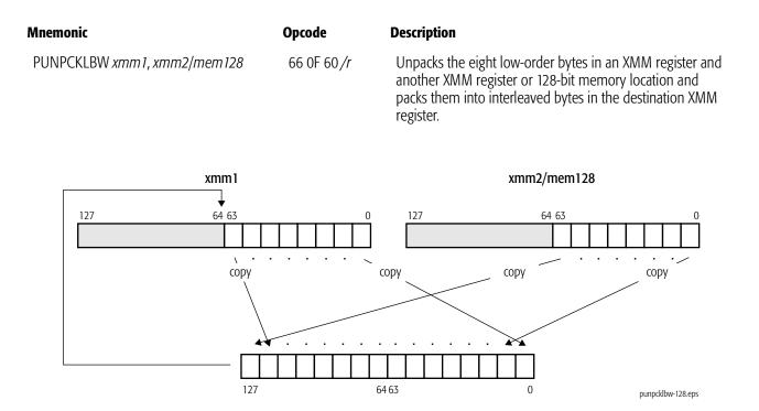
If the second source operand is all 0s, the destination contains the bytes from the first source operand zero-extended to 16 bits. This operation is useful for expanding unsigned 8-bit values to unsigned 16-bit operands for subsequent processing that requires higher precision.
