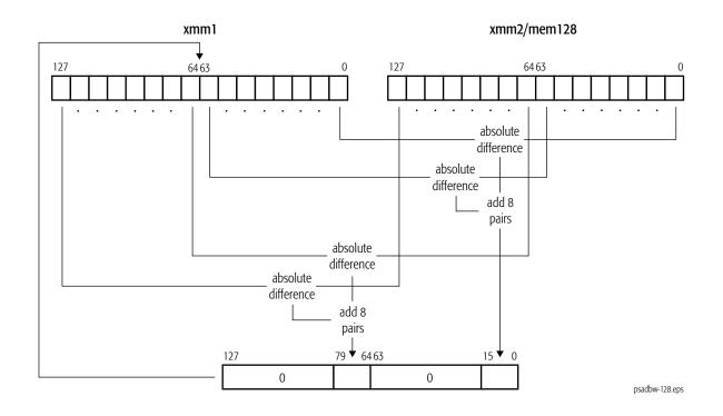
The sum of the differences of the eight bytes in the high-order quadwords of the source operands are written in the least-significant word of the high-order quadword in the destination XMM register, with the remaining bytes cleared to all 0s. The sum of
