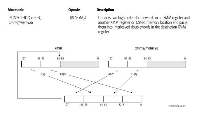
If the second source operand is all 0s, the destination contains the doubleword(s) from the first source operand zero-extended to 64 bits. This operation is useful for expanding unsigned 32-bit values to unsigned 64-bit operands for subsequent processing that requires higher precision.
