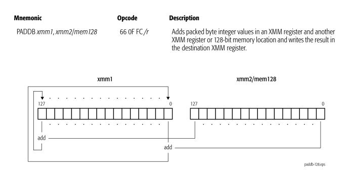
This instruction operates on both signed and unsigned integers. If the result overflows, the carry is ignored (neither the overflow nor carry bit in rFLAGS is set), and only the low-order 8 bits of each result are written in the destination.
