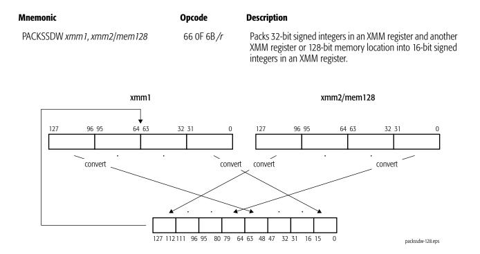
For each packed value in the destination, if the value is larger than the largest signed 16-bit integer, it is saturated to 7FFFh, and if the value is smaller than the smallest signed 16-bit integer, it is saturated to 8000h.
