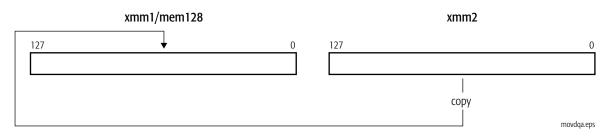
A memory operand that is not aligned on a 16-byte boundary causes a generalprotection exception.
