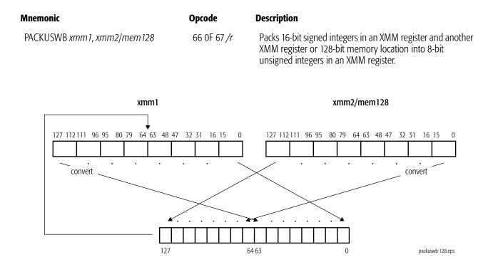
For each packed value in the destination, if the value is larger than the largest unsigned 8-bit integer, it is saturated to FFh, and if the value is smaller than the smallest unsigned 8-bit integer, it is saturated to 00h.
