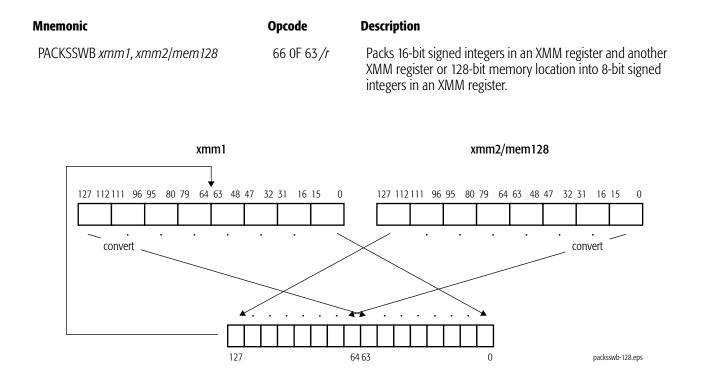
For each packed value in the destination, if the value is larger than the largest signed 8-bit integer, it is saturated to 7Fh, and if the value is smaller than the smallest signed 8-bit integer, it is saturated to 80h.
