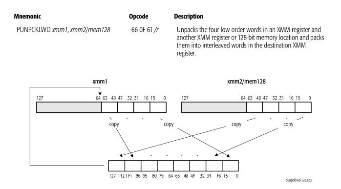
If the second source operand is all 0s, the destination contains the words from the first source operand zero-extended to 32 bits. This operation is useful for expanding unsigned 16-bit values to unsigned 32-bit operands for subsequent processing that requires higher precision.
