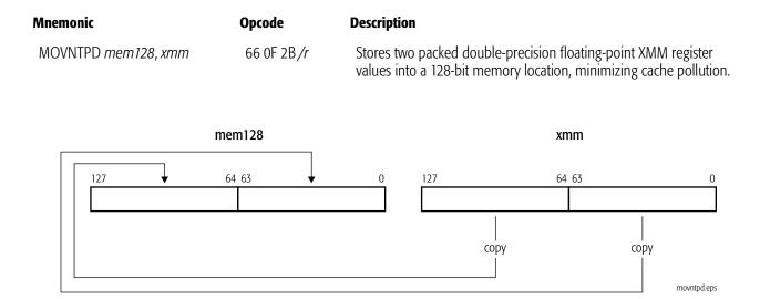
MOVNTPD is weakly-ordered with respect to other instructions that operate on memory. Software should use an SFENCE instruction to force strong memory ordering of MOVNTPD with respect to other stores.
