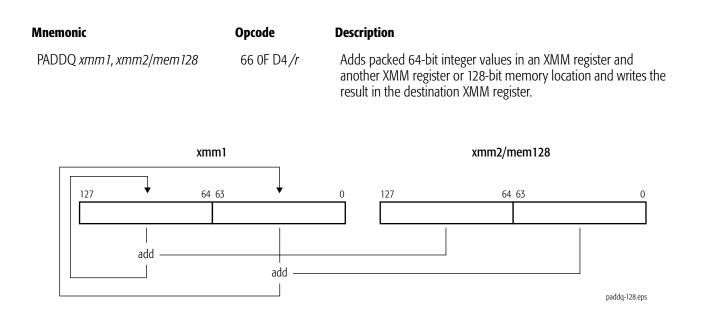
This instruction operates on both signed and unsigned integers. If the result overflows, the carry is ignored (neither the overflow nor carry bit in rFLAGS is set), and only the low-order 64 bits of each result are written in the destination.
