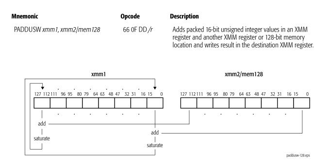
For each packed value in the destination, if the value is larger than the largest unsigned 16-bit integer, it is saturated to FFFFh, and if the value is smaller than the smallest unsigned 16-bit integer, it is saturated to 0000h.
