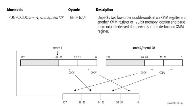
If the second source operand is all 0s, the destination contains the doubleword(s) from the first source operand zero-extended to 64 bits. This operation is useful for expanding unsigned 32-bit values to unsigned 64-bit operands for subsequent processing that requires higher precision.
