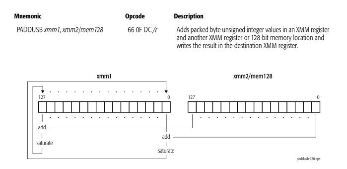
For each packed value in the destination, if the value is larger than the largest unsigned 8-bit integer, it is saturated to FFh, and if the value is smaller than the smallest unsigned 8-bit integer, it is saturated to 00h.
