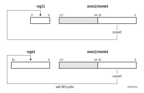
If the result of the conversion is an inexact value, the value is truncated (rounded toward zero). If the floating-point value is a NaN, infinity, or if the result of the conversion is larger than the maximum signed doubleword  $(-2^{31} \text{ to } +2^{31} - 1)$  or quadword value  $(-2^{63} \text{ to } +2^{63} - 1)$ , the instruction returns the indefinite integer value
