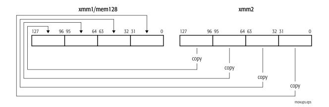
Memory operands that are not aligned on a 16-byte boundary do not cause a generalprotection exception.
