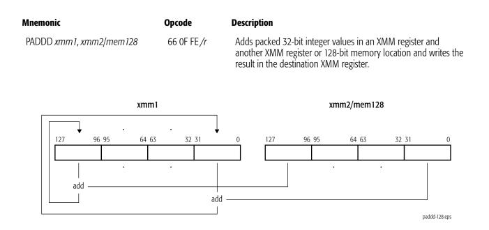
This instruction operates on both signed and unsigned integers. If the result overflows, the carry is ignored (neither the overflow nor carry bit in rFLAGS is set), and only the low-order 32 bits of each result are written in the destination.
