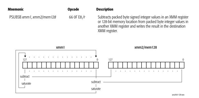
For each packed value in the destination, if the value is larger than the largest signed 8-bit integer, it is saturated to 7Fh, and if the value is smaller than the smallest signed 8-bit integer, it is saturated to 80h.
