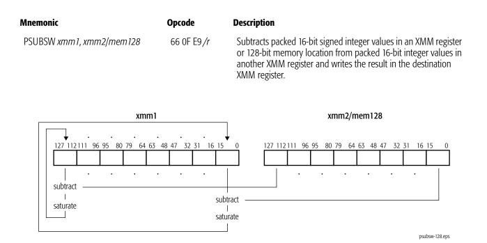
For each packed value in the destination, if the value is larger than the largest signed 16-bit integer, it is saturated to 7FFFh, and if the value is smaller than the smallest signed 16-bit integer, it is saturated to 8000h.
