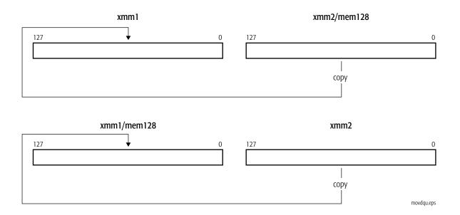
Memory operands that are not aligned on a 16-byte boundary do not cause a generalprotection exception.
