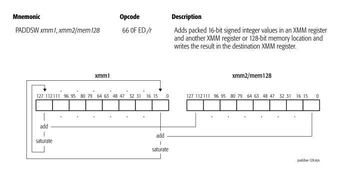
For each packed value in the destination, if the value is larger than the largest representable signed 16-bit integer, it is saturated to 7FFFh, and if the value is smaller than the smallest signed 16-bit integer, it is saturated to 8000h.
