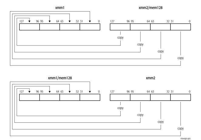
A memory operand that is not aligned on a 16-byte boundary causes a generalprotection exception.
