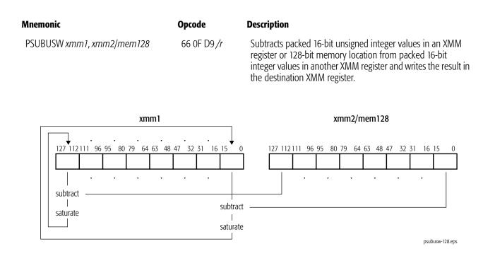
For each packed value in the destination, if the value is larger than the largest unsigned 16-bit integer, it is saturated to FFFFh, and if the value is smaller than the smallest unsigned 16-bit integer, it is saturated to 0000h.
