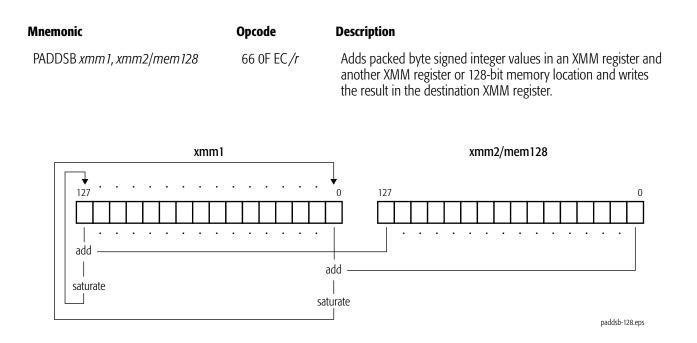
For each packed value in the destination, if the value is larger than the largest representable signed 8-bit integer, it is saturated to 7Fh, and if the value is smaller than the smallest signed 8-bit integer, it is saturated to 80h.
