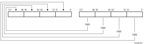
MOVNTPD is weakly-ordered with respect to other instructions that operate on memory. Software should use an SFENCE instruction to force strong memory ordering of MOVNTPD with respect to other stores.
