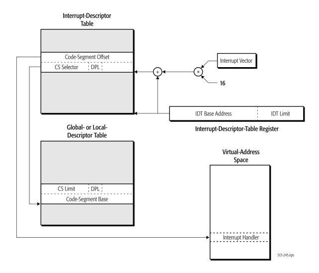
Figure 8-12. Long-Mode Interrupt Control Transfer
