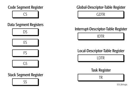
Figure 4-2. Segment and Descriptor-Table Registers
