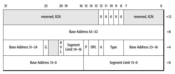
Figure 4-22. System-Segment Descriptor–64-Bit Mode
