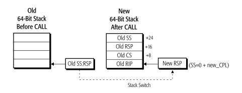
Figure 4-35. Stack Switch–Long Mode
