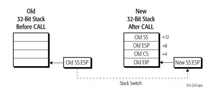
Figure 4-34. 32-Bit Stack Switch, No Parameters–Legacy Mode
