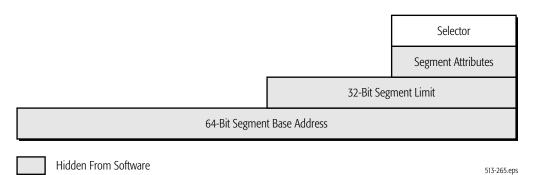
Figure 4-5. FS and GS Segment-Register Format–64-Bit Mode
