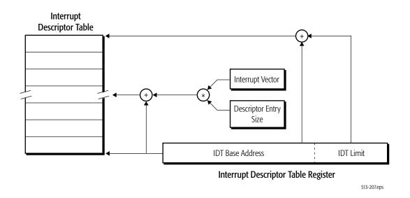
Figure 4-12. Indexing an IDT
