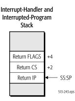
Figure 8-6. Stack After Interrupt in Real Mode
